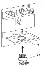
A. Removable retaining nut B. Strain relief
